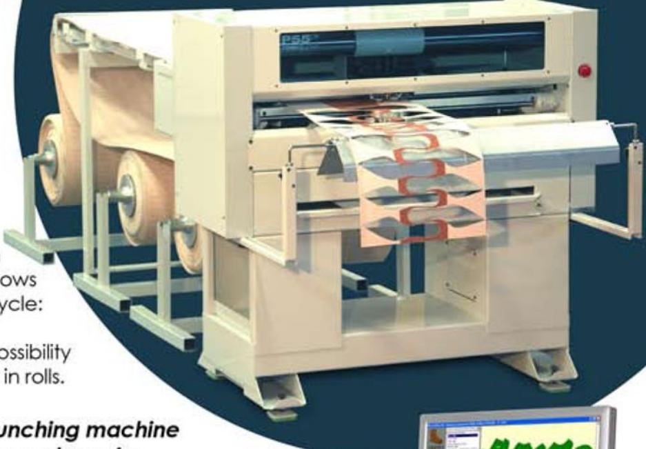
*P55 is therefore an "automatic" punching machine that eliminates dead time and does not require constant presence of the operator to remove pieces and waste or for frequent loading of the material.*
